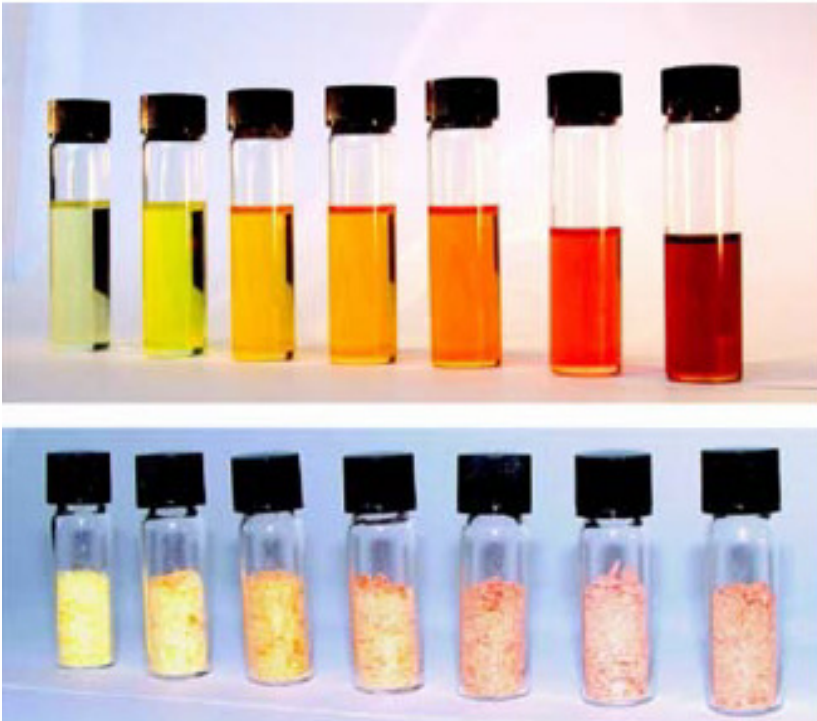
Various size of CdSe nanoparticles and their solution. The bulk CdSe is black
